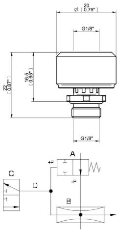
A=AQR, B=Vacuum pump, C=Control valve, D=Rec. max. 1.5m
