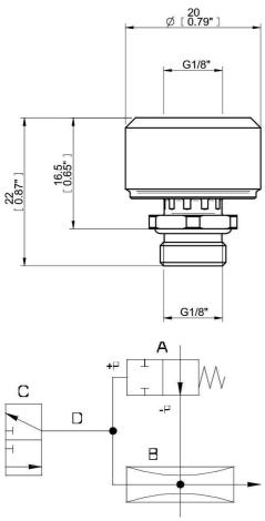
A=AQR, B=Vacuum pump, C=Control valve, D=Rec. max. 1.5m
