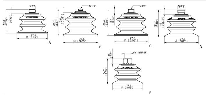
Suction cup BX75P Polyurethane 60 with filter, brass 3/8" NPSF female
